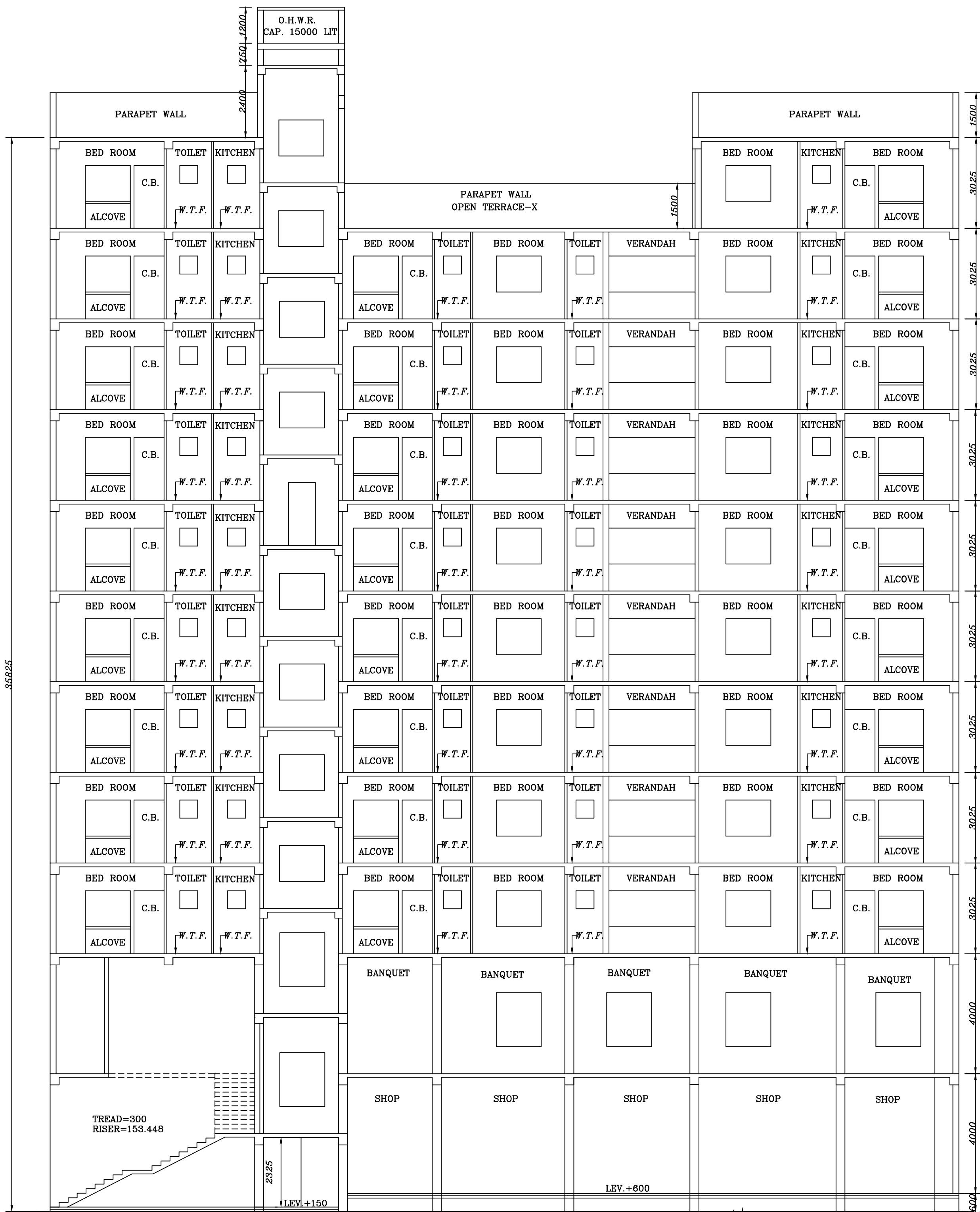
SECTION AT -"A-A" SCALE:1:100
